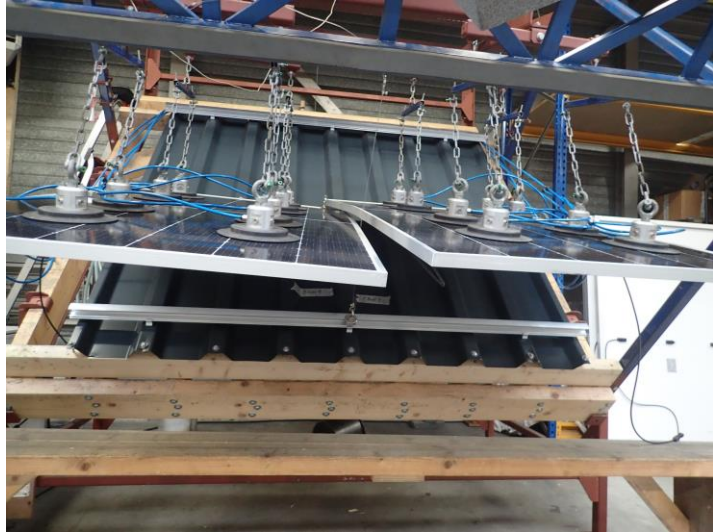
Photo 10 Detail of the failure mode of test specimen 1.
