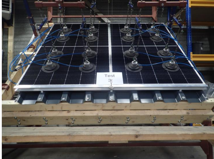
Photo 13 The suction cups are placed in position and test specimen 3 is ready for testing.
